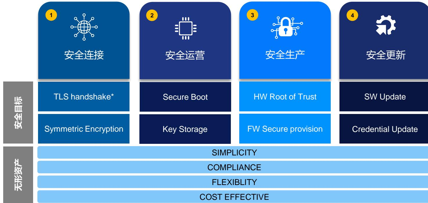
TLS handshake\* : HW pre-integration of common SSL stacks e.g OpenSSL, mbedTLS..
