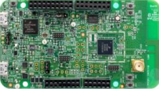
This page documents a pre-configured FreeRTOS Eclipse/GCC project that targets a RISC-V core on the RV32M1 VEGAboard. The RV32M1 incorporates a PULP RI5CY RISC-V core, a PULP Zero RISCY RISC-V core, an Arm Cortex-M4 core, and an Arm Cortex-M0+ core. At the time of writing this demo only targets the RI5CY RISC-V core.
