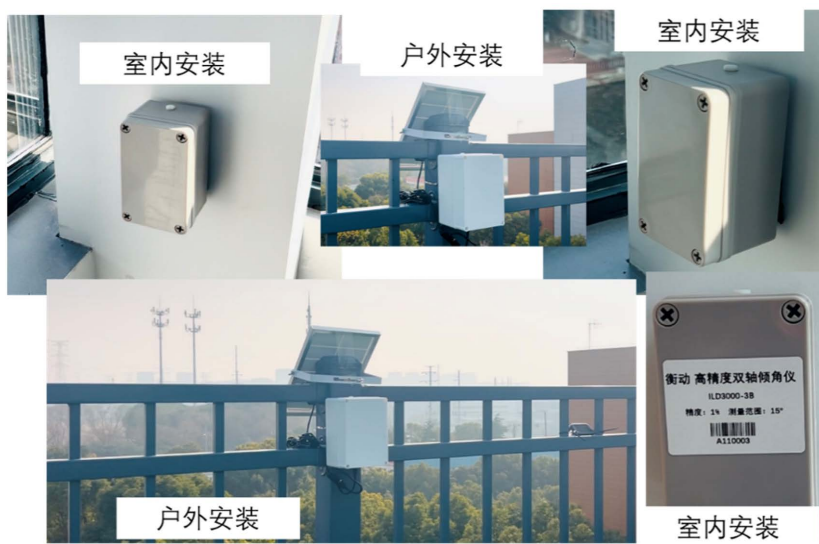
Figure 11. Installation diagram of Low-Power 4G and Wi-Fi stability testing product 图 11. 低功耗 4G 和 Wi-Fi 稳固测试产品安装图片
