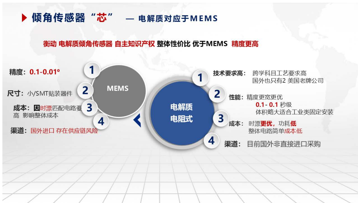
Figure 5. Performance and cost-effectiveness comparison between electrolyte and MEMS tilt sensors 图 5. 倾角传感器性能电解质对比于 MEMS 性价比图片
