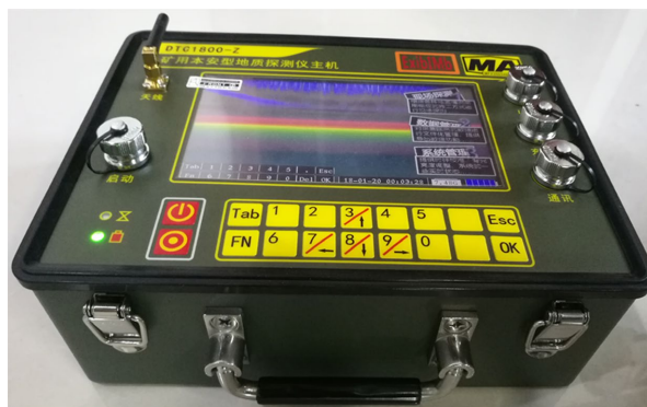
Figure 2. Appearance diagram of the wireless host in the high-precision borehole seismic prediction system for tunnel excavation 图 2. 巷道掘进中孔中地震高精度预报系统无线主机外观示意图
