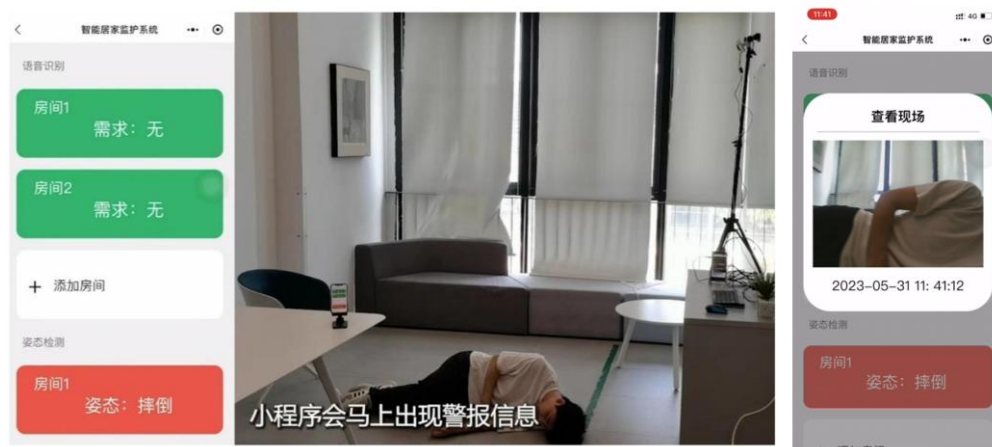
Figure 13. Detecting a person's fall and issuing an alarm through millimeter wave radar
