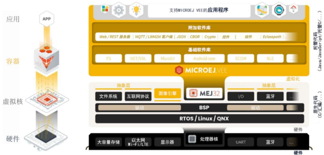
Figure 5. A small real-time container solution: MICROEJ VEE
